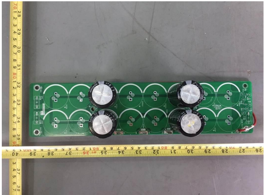
Back View of Hiverter Si-50K Cap. board
